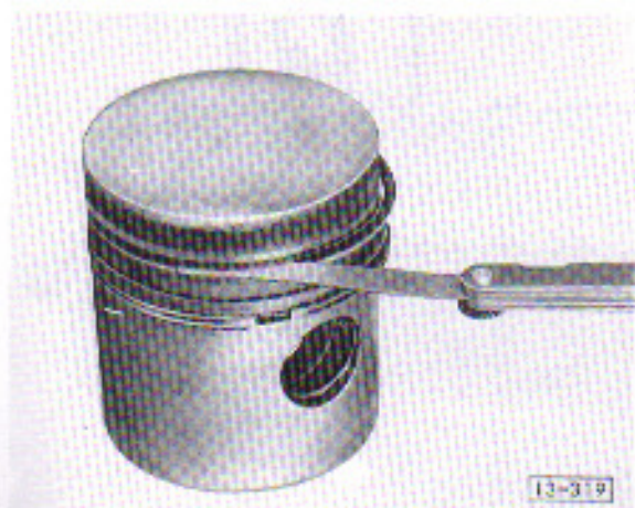
Fig. 7 Piston rings – Checking side clearance
