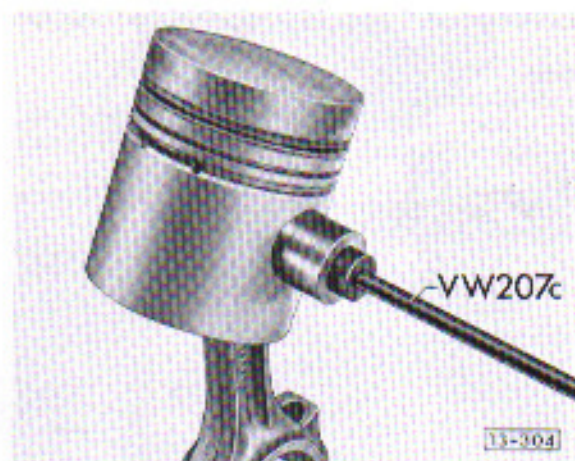
Fig. 3 Piston pins – Removing and installing AUDI: Piston pin mandrel 10-508.
