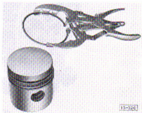
Fig. 5 Pistons rings – Removing and installing "Top" must be upwards.
