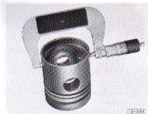
Fig. 10 Pistons – Checking
