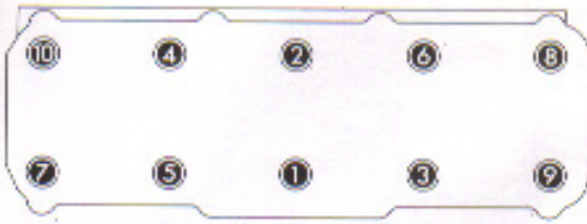
Fig. 1 Removing and installing cylinder head
