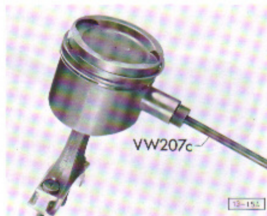
Fig. 5 Removing and installing piston pins
