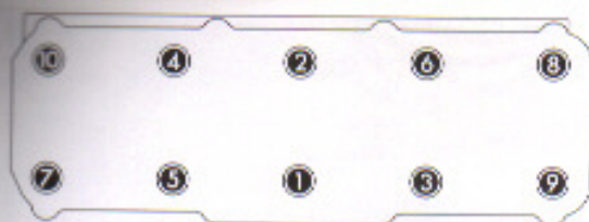
Fig. 1 Removing and installing cylinder head
